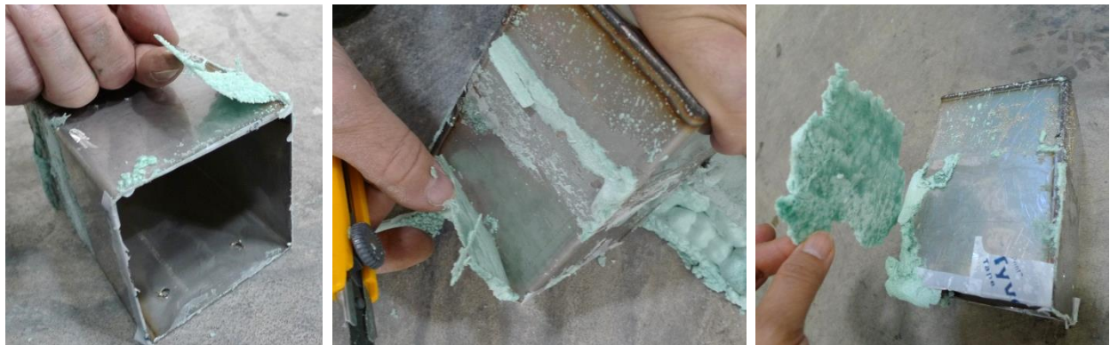
Figure 37. Foam easily detached from ducts that were sprayed with silicone.
