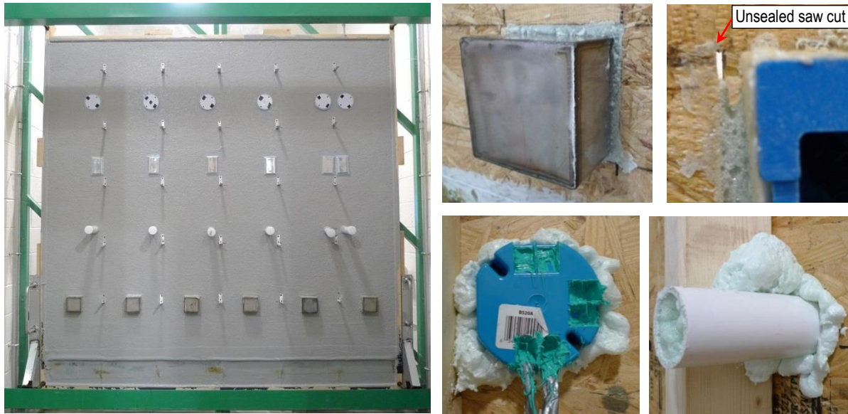
Figure 30. Test wall with fluid-applied membrane as the air barrier material.
