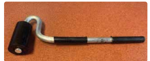
ABAA Roller Provided to Accredited Contractors
