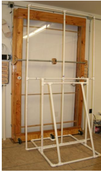
Figure 9. Test wall pressurization setup.
