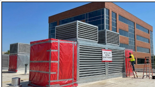
Photo 1: Building Envelope Test: Sealing off the HVAC to test Building Envelope Material Installation
